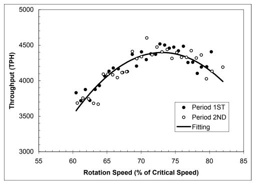
Figure 5. Maximizing Throughput for Rotation Speed
