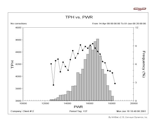
Figure 3. Throughput vs. SAG Power Draw
