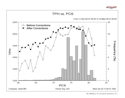
Figure 13. Throughput vs. Rotation Speed (% of Critical)
