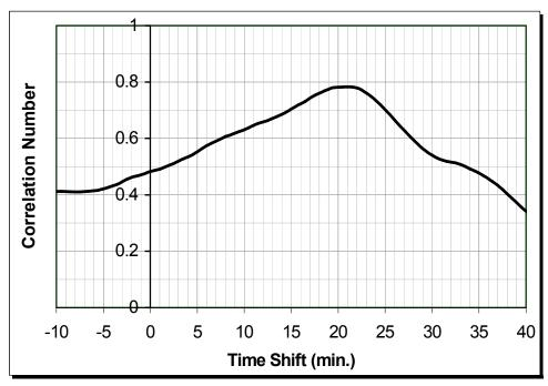
Fig. 15: Phase Shift between Circuit Feed Rate and Product Size
