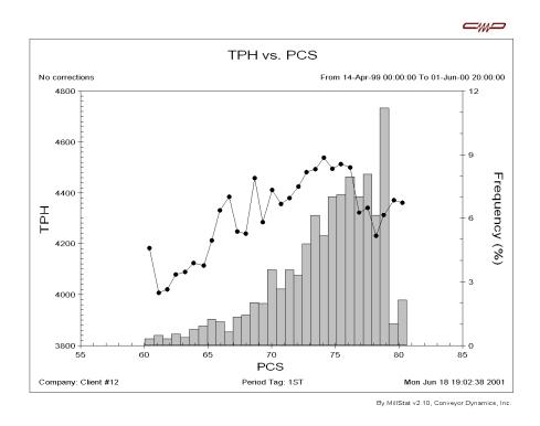
Figure 4. Throughput vs. Rotation Speed (% of Critical)
