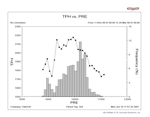
Figure 1. Throughput vs. Bearing Pressure
