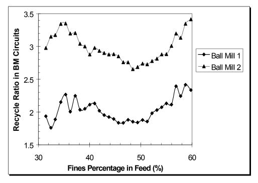
Figure 10. Recycle Ratio in BM Circuits vs. Fines Percentage in Feed
