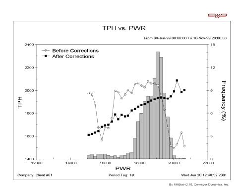
Figure 11. Throughput vs. SAG Power for 1st Period
