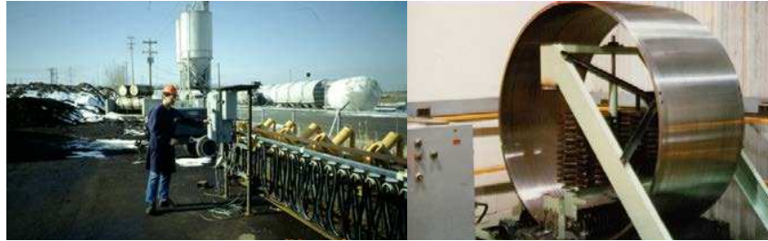
Fig. 2: CDI's model validation test machines: trampling and flexure loss test machine (left); indentation loss test machine (right)
