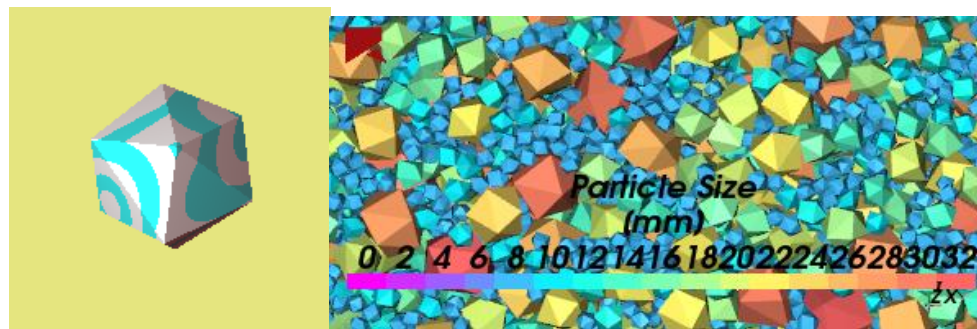
Figure 11: Particle Shape and Size with 10 facets left; at right is Table 2 PSD used for HPGR and CAHM simulations – yields a highly competent ore vs. a more slabby ore
