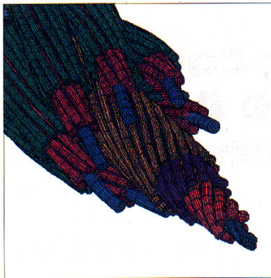
Fig. 1: Wire rope construction - Palabora ST 6600 N/mm belt with 12.4 mm diameter cable
