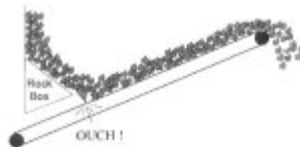
FIGURE 1: TYPICAL HARD ROCK BOX
